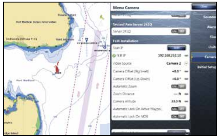
The NavNet TZtouch displays custom settings for the camera, including zoom distance, camera altitude, and automatic locking on an active waypoint or Man Over Board (MOB).
