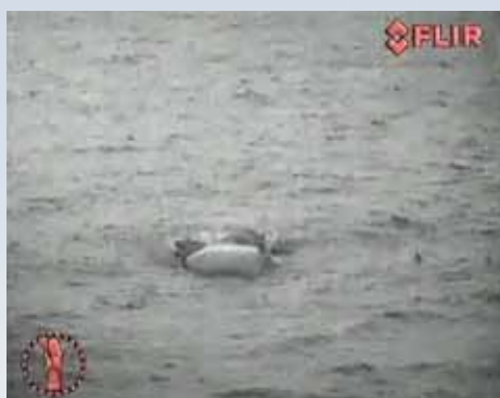
With the thermal imaging camera very small growlers can be detected from distances of over 800 meters.
