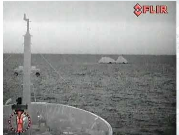
The searchlight only illuminates objects in the narrow path of its lightbeam. A thermal imaging camera presents a much wider view, resulting in better situational awareness.
