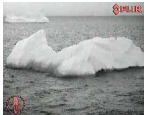
The narrow beam of the searchlight needs to be pointed directly at this bergy bit to illuminate it.
